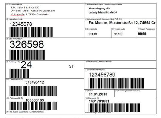
Sample of a goods label according to VDA 4902 with bar code 128
