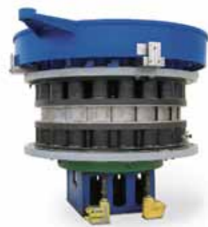
Refurbished distributor for a 38 MW vertical Francis turbine.
