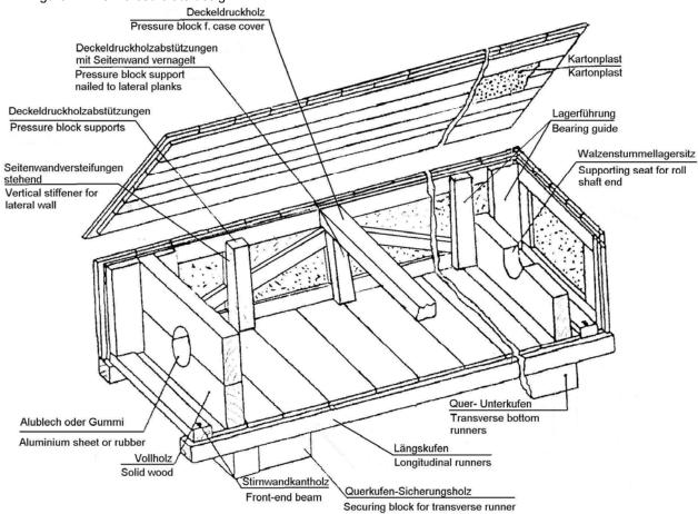
Figure 13: Crate design (roll bearing)
