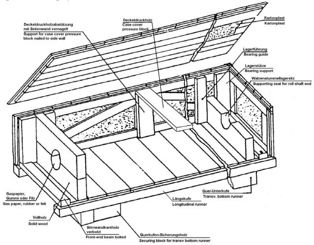
Figure 11: Crate design (roll bearing) from 3 t
