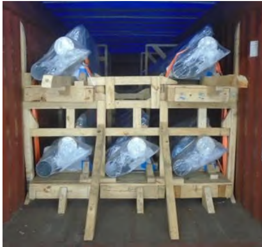
Figure 15: Example of packaging and securing multiple components on top of one another in the container without separate crate
