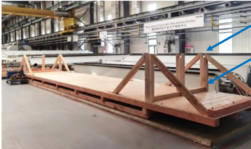
Figure 7: Example for wood pallet with frame
