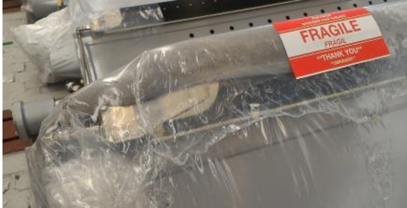
Figure 5: Example for specific marking of sensitive areas
