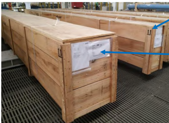
Figure 12: Example of packaging in wooden crate with handling marking and labeling
