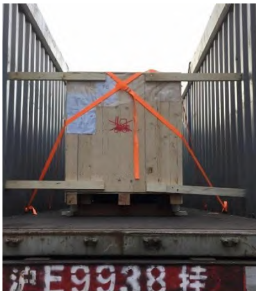
Figure 13, 14: Example of fixation crate in container
