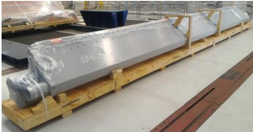
Figure 6: Example for storage on a wooden floor
