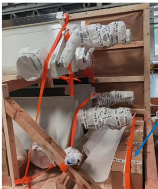
Figure 9: Example of fixation with belts
