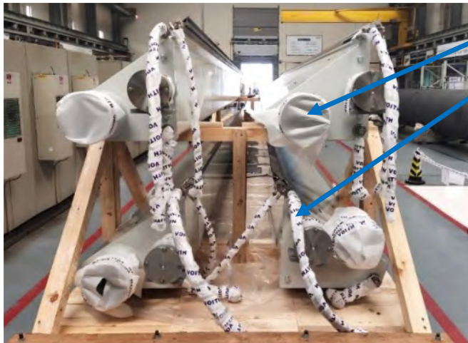
Figure 8: Example of multiple doctor layers loaded onto pallet
