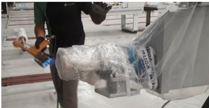
Figure 4: Example for protection in the bearing area with shrink foil
