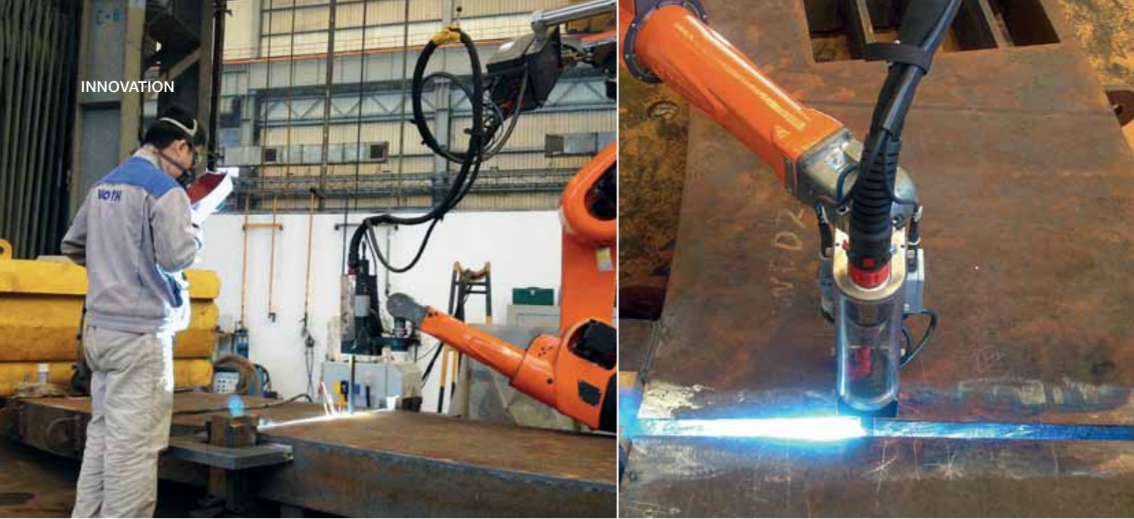
Narrow gap welding at the Voith Hydro workshop in Shanghai.
