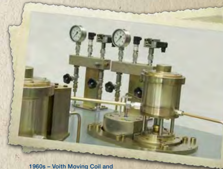
1960s – Voith Moving Coil and additional control equipment.
