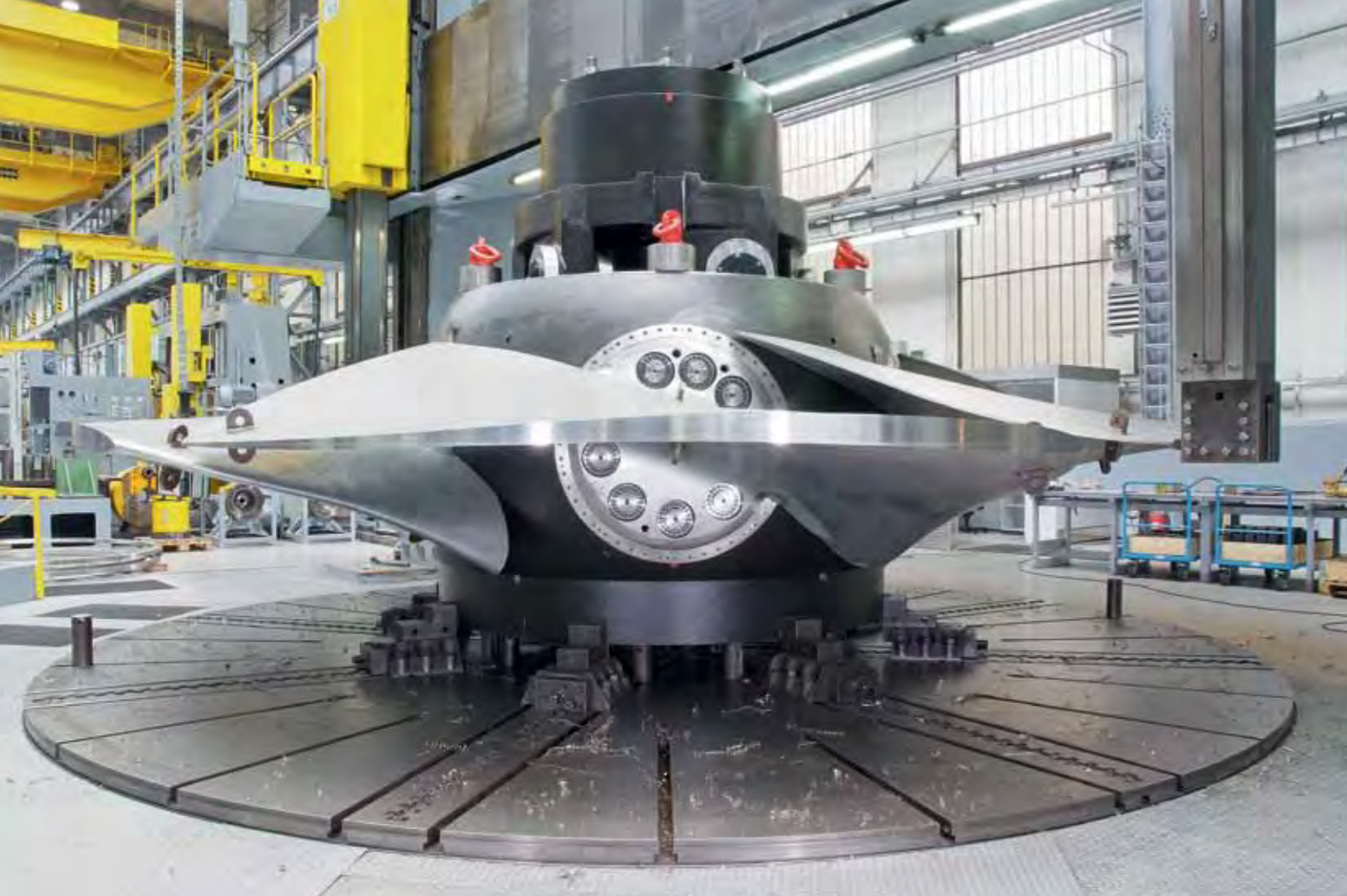
Kaplan turbine at the Voith Workshop in Heidenheim, Germany.
