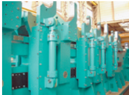
Fig. 1: Janus™ MK 2 with un- and rewind section including flying splice.
