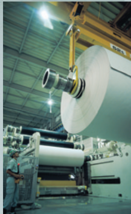
Fig. 4: Sirius reel with 4 m parent roll.
