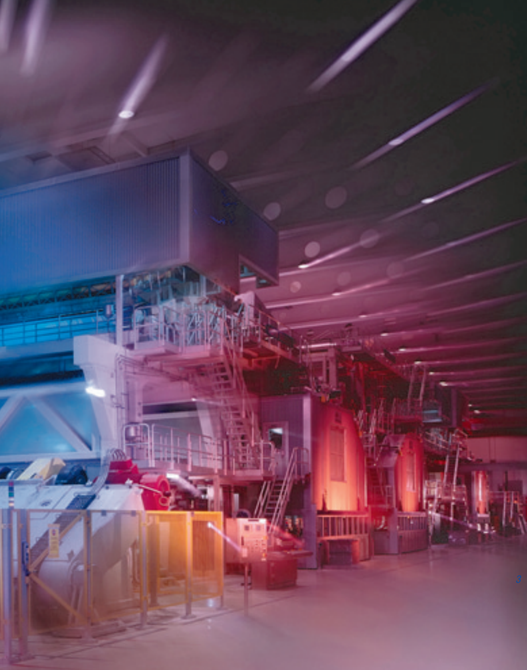
Fig. 3: The coating machine produces 2,735 t/24 h of Magno Matt grades at 150 and 170 g/m 2 .
