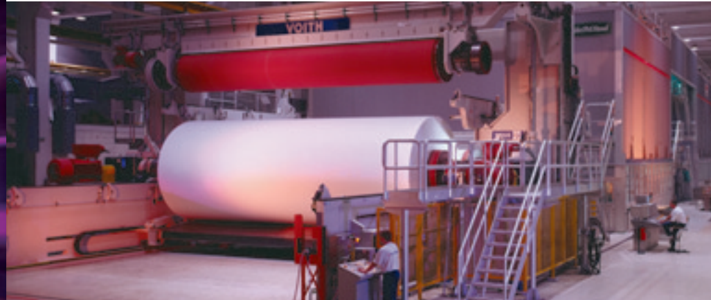
Fig. 2: The paper machine output is 1,732 t/24 h.
