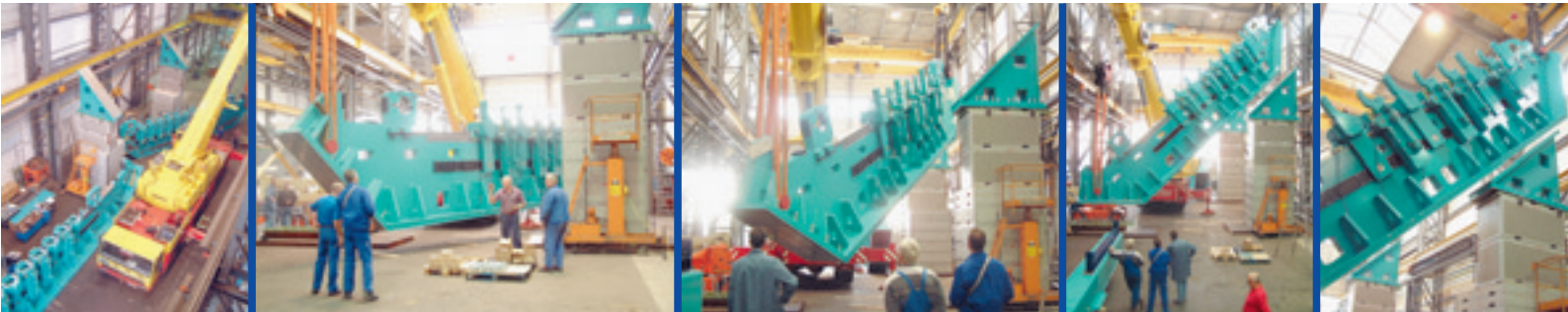
For detecting any interference points, the frames and upper cross beams were precisely aligned in exactly the same way as they would be on-site. Subsequently, the inner traverse platforms, the pipe racks on both the drive and tender sides and the fixed or movable stairways on both sides were assembled (Fig. 5).
