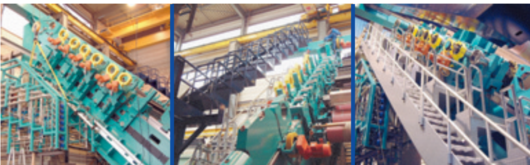
For detecting any interference points, the frames and upper cross beams were precisely aligned in exactly the same way as they would be on-site. Subsequently, the inner traverse platforms, the pipe racks on both the drive and tender sides and the fixed or movable stairways on both sides were assembled (Fig. 5).
