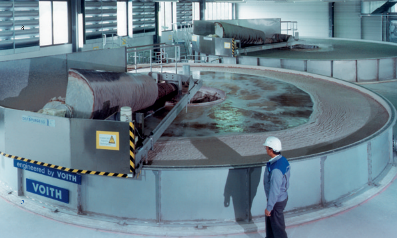
Fig. 3: The two DeltaPurge micro-flotation units supplied by Voith Paper's joint venture partner Meri; in the foreground for Loop II, in the background for Loop I.
