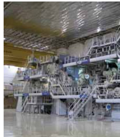
Wet end with DuoFormer TQv and Tandem NipcoFlex press.
