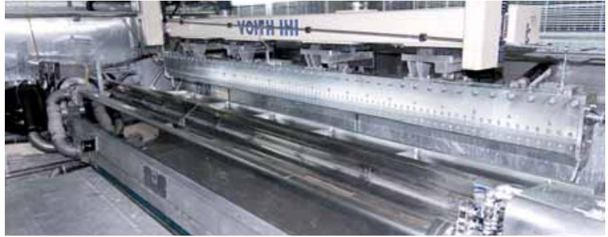
Due to higher solids content of the coating color, energy in the drying section can be saved.
