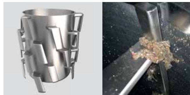
Asia results case study with MultiFoil. The right picture shows a rotor of a non-Voith TLA 450 screen with spinnings at the foil blades.
