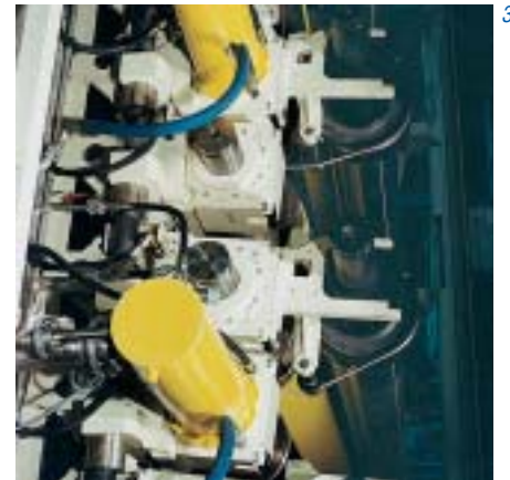
Fig. 4: Calender unwind system.
