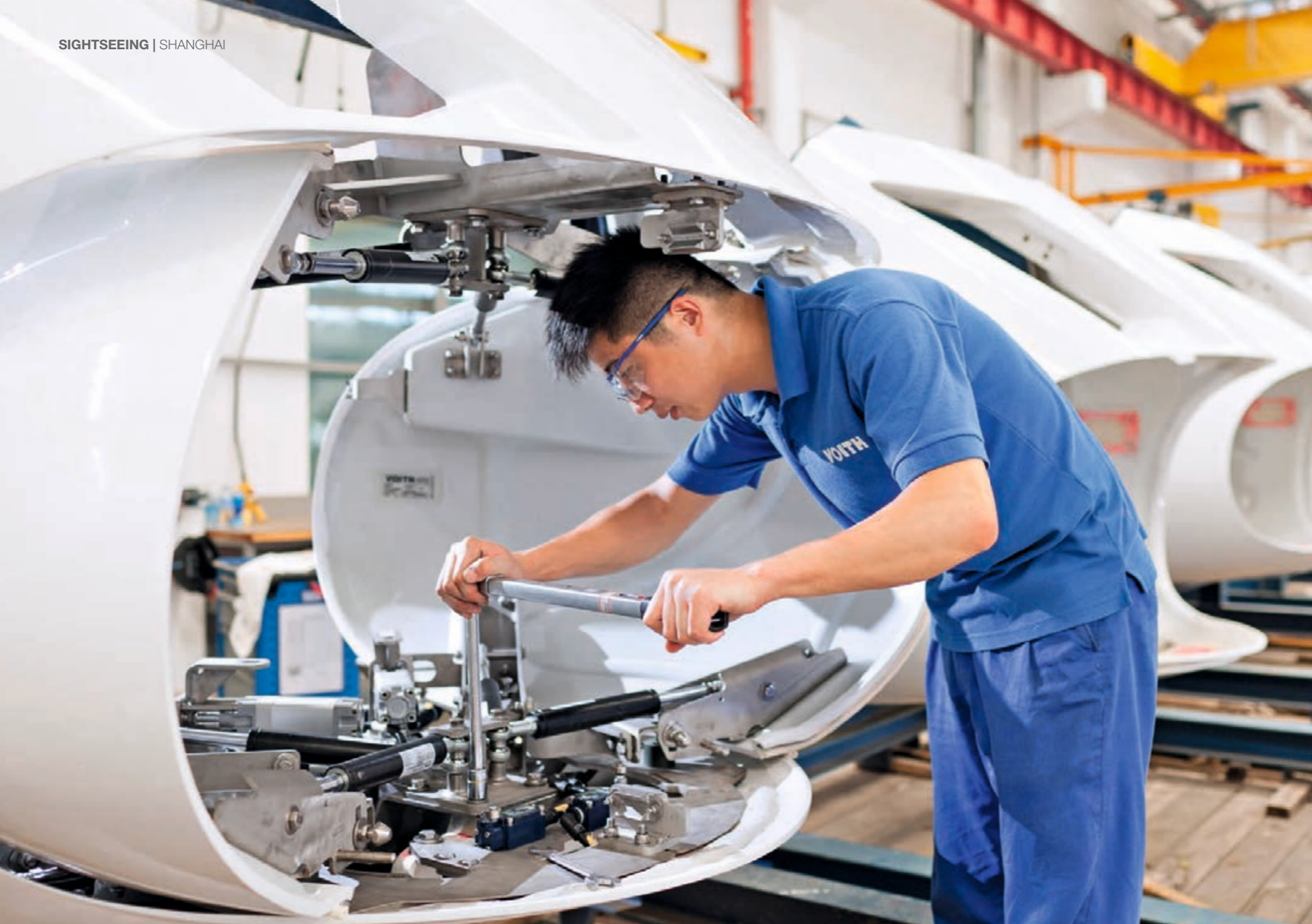
Precision – for maximum safety: Work in the Voith plant in Shanghai on front ends for high-speed trains in China.
