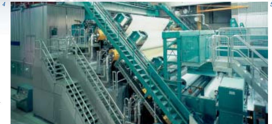
Fig. 5: Janus MK 2 in operation. A photograph of a Janus MK 2 calender machine in operation, showing the paper web being processed by multiple rollers.
