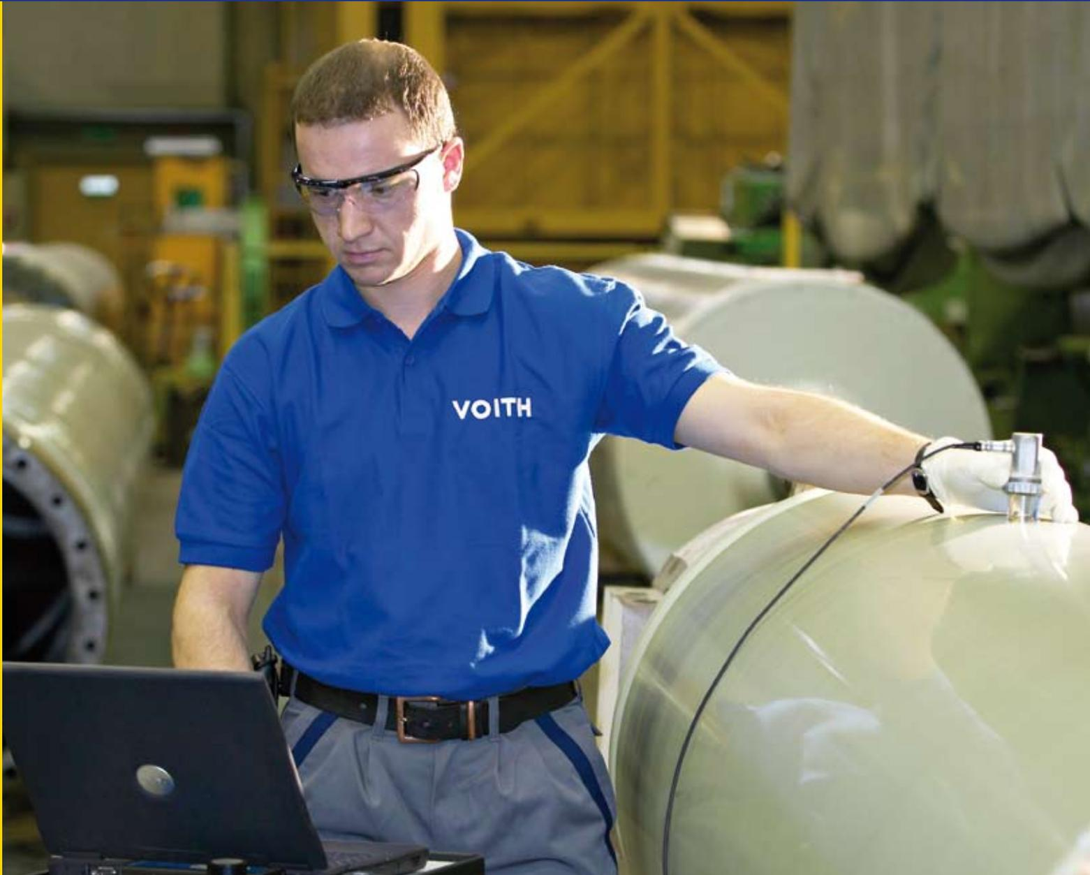
*RollCare: Ultrasonic testing of a roll cover.*
