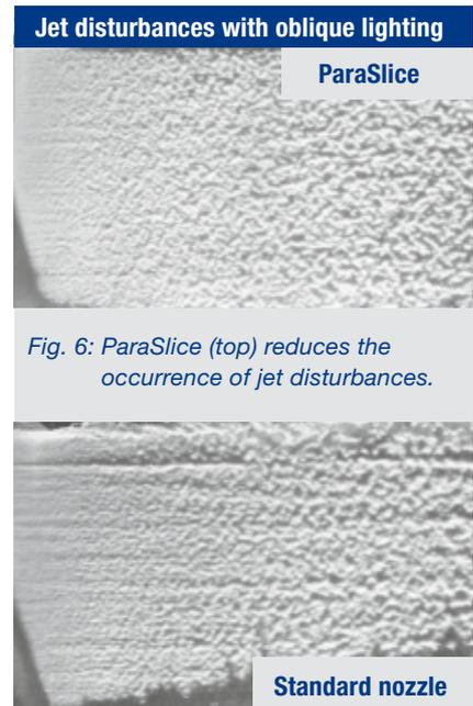
Fig. 6: ParaSlice (top) reduces the occurrence of jet disturbances.
