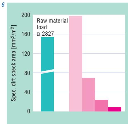
must be achieved using two additional flotation modules. This method of extrapolating the results is illustrated in Fig. 6.
