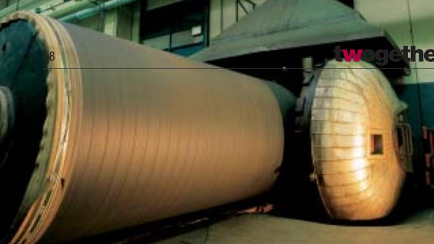
Fig. 3: Forming roll covered with Diamantite put into the curing chamber for Andritz AG, size of the roll: 1500 x 1512 x 3300 mm.
