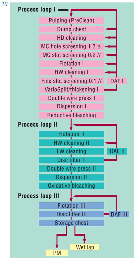
Fig. 8: Process arrangement used for the pilot trials.
