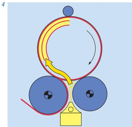
a single drum winder had to be used. The reason for this were the nip forces resulting from the great roll weights which, with the two drum winder, could lead to winding faults, such as crepe wrinkles, breakages, excessive stretch etc. Fig. 3 shows an example of 2 types of paper on this subject.
