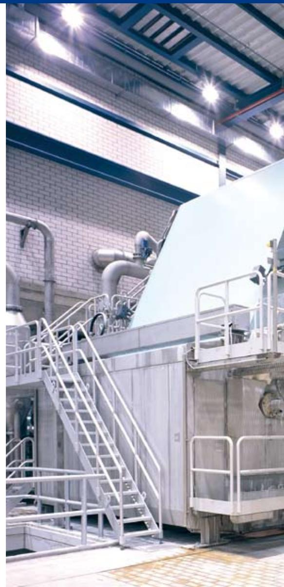
liquid curtain to the paper web. In order to reduce curling that occurs for papers with one-sided coating (warping in the paper), each of the two coating machines were equipped with a ModulePro C jet spray applicator system in 2006. The ModulePro C compensates for the roll tendency of the paper by releasing frozen warps that remoisten the web on the non coated side. The new technology
