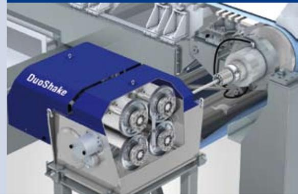
*For décor paper machines Voith Paper uses the MasterJet headbox in conjunction with the EdgeModule edge feed-in system to achieve optimum fiber orientation at the web edge. The DuoShake shaker ensures a particularly homogeneous distribution of the fibers in the sheet.*
