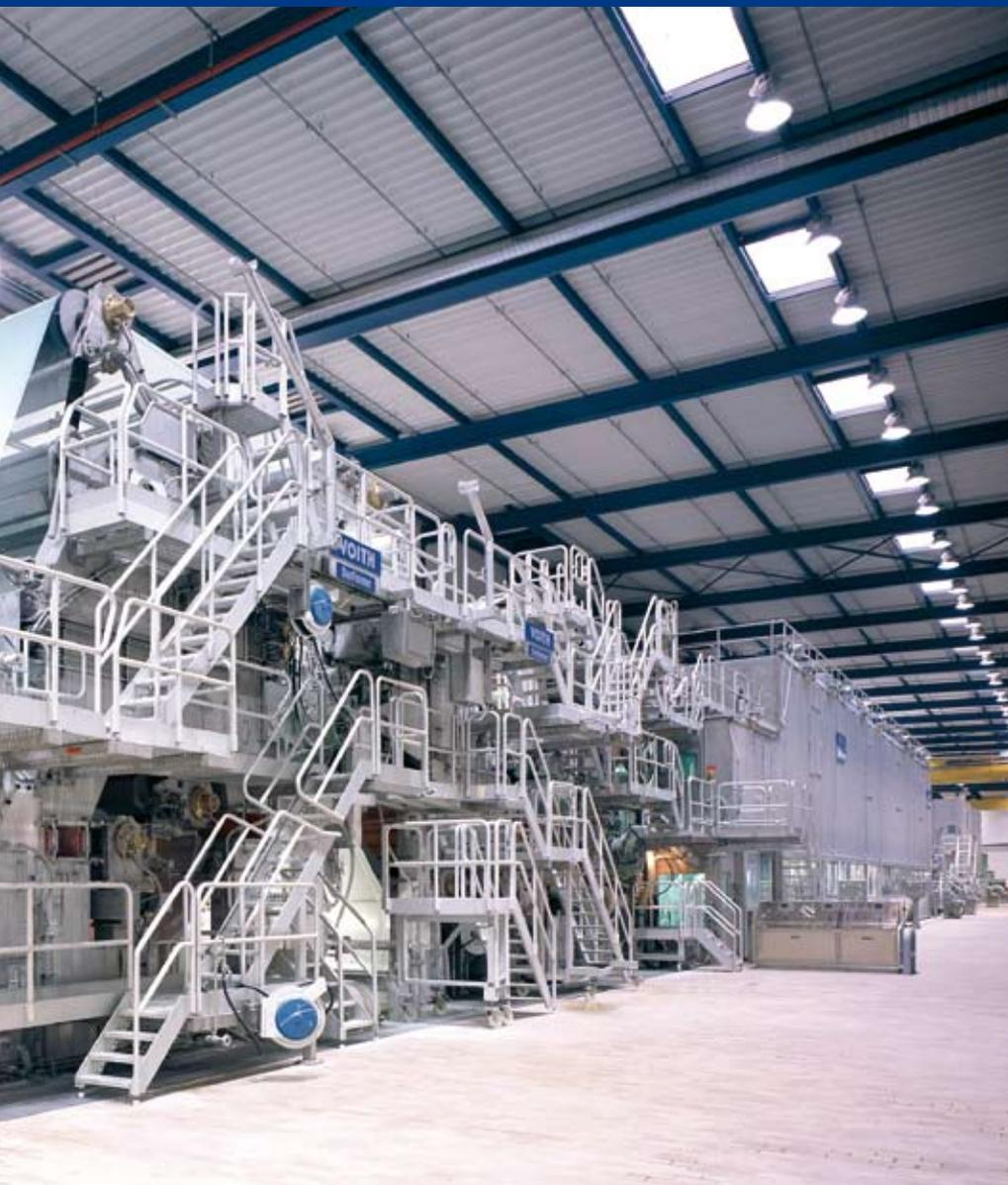
*The PM 2 at the Koehler facilities in Kehl is used exclusively for the production of thermo papers in the basis weight range of 40 to 80 g/m<sup>2</sup> and at a production speed of 1,600 m/min.*
