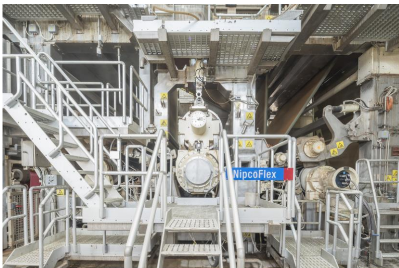
Caption picture 1: Voith NipcoFlex shoe press at Macedonian Paper Mills BM1
