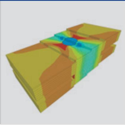
Figure 10: Nonlinear stress-strain analysis of a periodic segment of a rotor rim for homogenized FE analysis.
