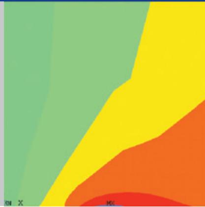
Figure 9: Electric potential at a semi-conductive corona protection of the stator end winding.
