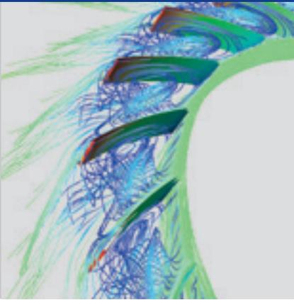
Figure 8: CFD analysis of a radial fan.
