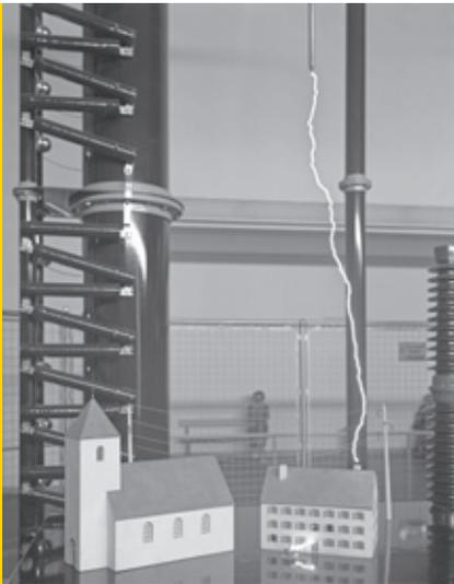
*Lightning model in the high-voltage apparatus.*
