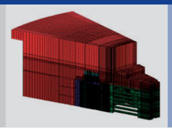
Figure 1: Solid geometry meshed for thermal analysis.
