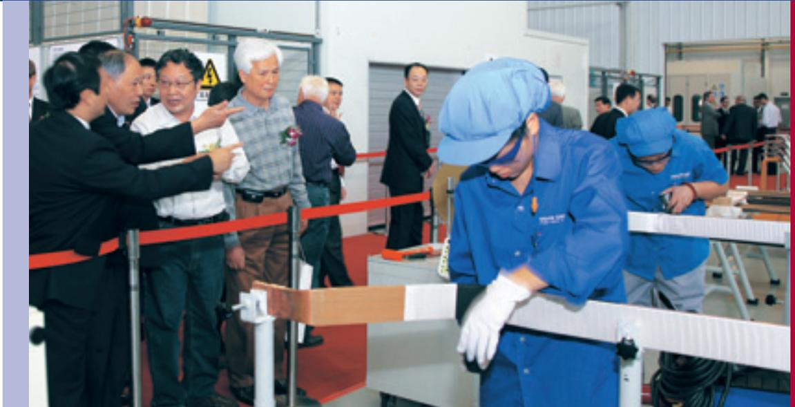
*During the opening festivities in Shanghai, employees demonstrate insulation of stator bars which is the heart of stator bar manufacturing.*
