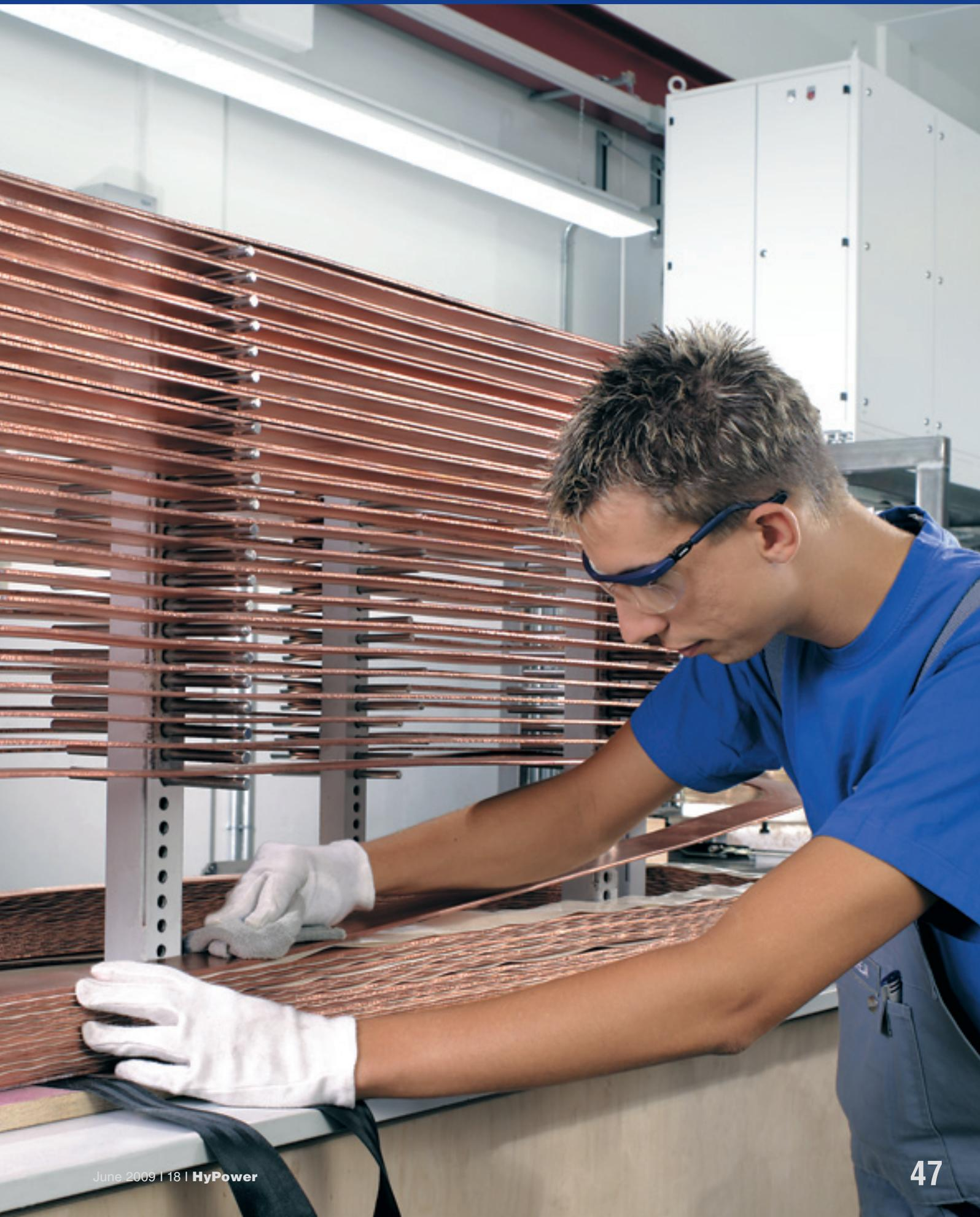
The expansion of the generator workshop took place in two steps. The first step was to implement a new work area for the rehabilitation of generator stators and rotors. Heart of the workshop is a 1,000 tons press which is an in-house development for the manufacturing of rotor coil windings. Stacking of new stator cores, assembly of stator windings and re-insulation of poles was feasible from spring 2007 on.
