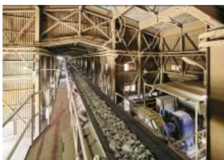
The combination of Voith hydrodynamic couplings and the respective control system allows for optimized operational characteristics of the conveyor and an increased belt lifetime.
