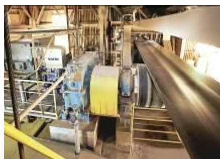
The combination of Voith hydrodynamic couplings and the respective control system allows for optimized operational characteristics of the conveyor and an increased belt lifetime.
