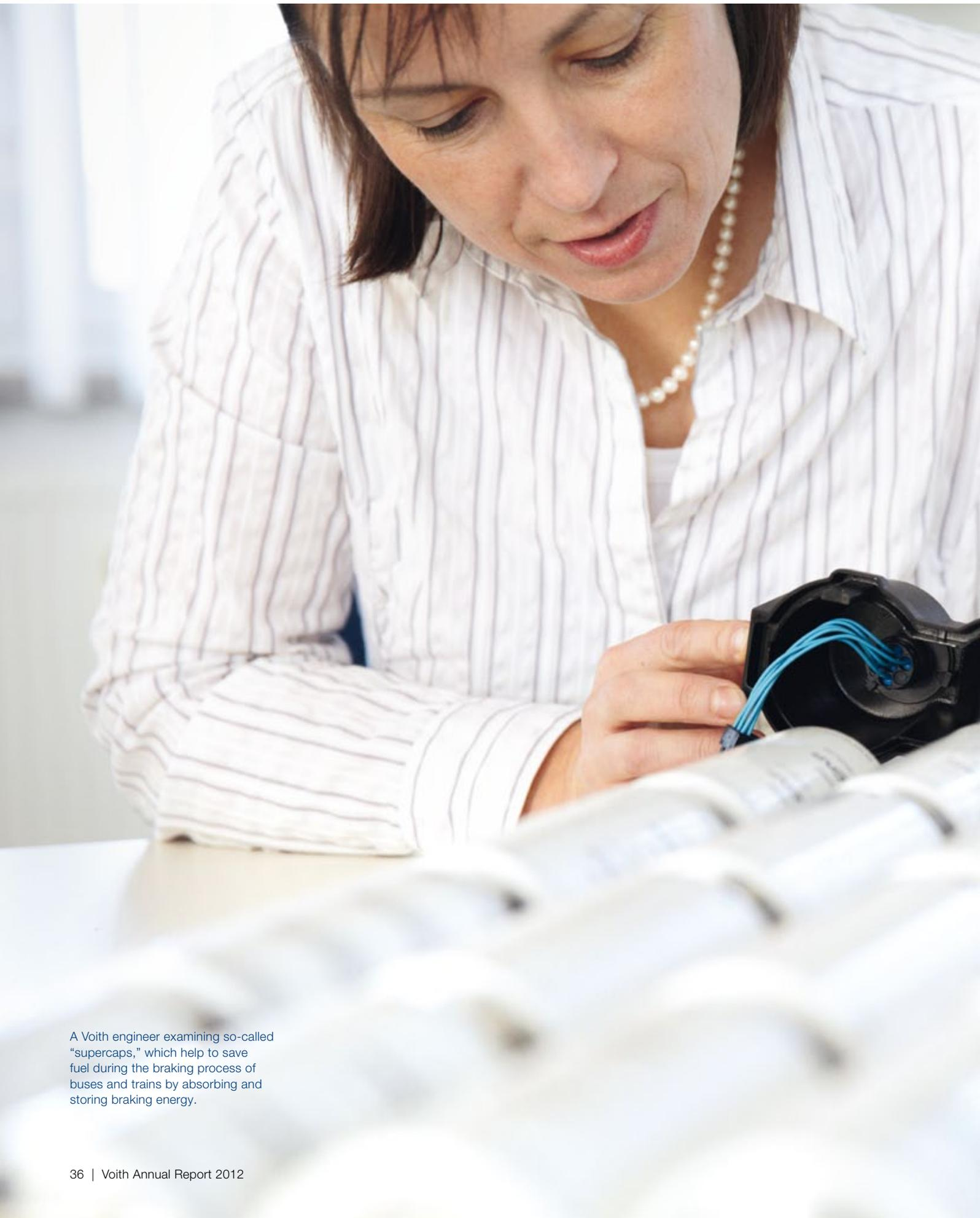
A Voith engineer examining so-called “supercaps,” which help to save fuel during the braking process of buses and trains by absorbing and storing braking energy.
