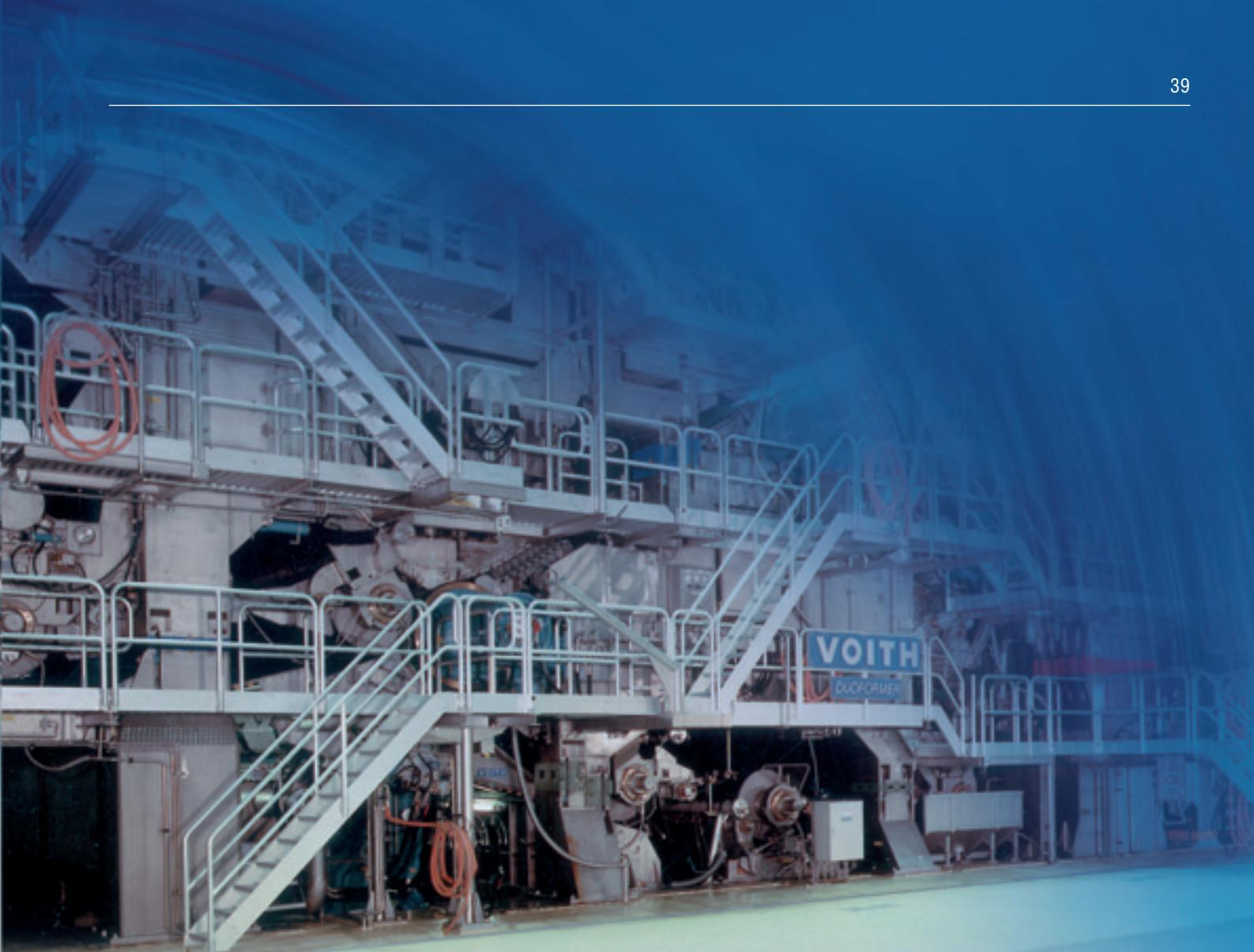
groups. The steam and condensate system was modified, and the fixed doctor blade holders were converted to flexible ones. At the end of 2001 a scanner with moisture sensor was installed.
