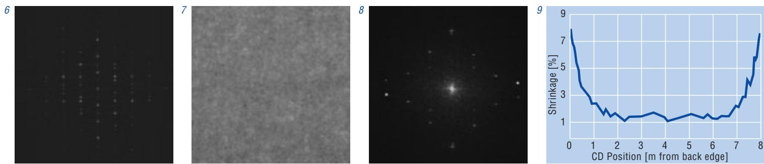
the peaks selected in *Fig. 4* are clearly also found in *Fig. 6* confirming that this forming fabric is the source of the mark in the paper, and not a press fabric as was thought by the papermaker.
