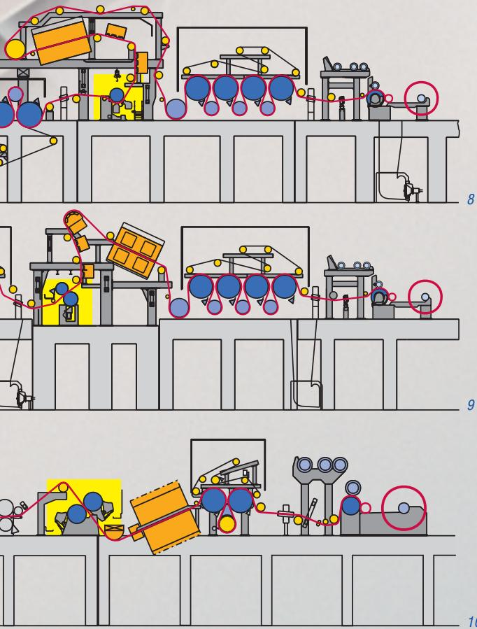
Fig. 8: Machine concept Offline Coater.
