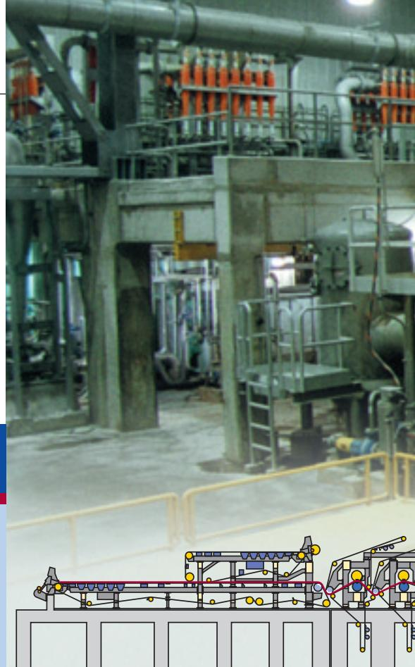
In terms of technology, the new mill is able to clean and fractionate fibers, by separating long from short fibers, in order to treat them differently, without any damage, thus obtaining a higher strength level at lower basis weight. Due to the project modernization level, all contaminants from treatment plants are removed in a solid and compact way. In addition, the noise level and water consumption are reduced, and the plant is ISO 14000 certified.
