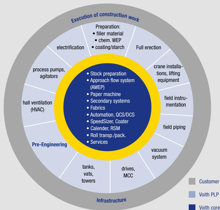
Fig. 3: Typical supply limits with PLP projects.
