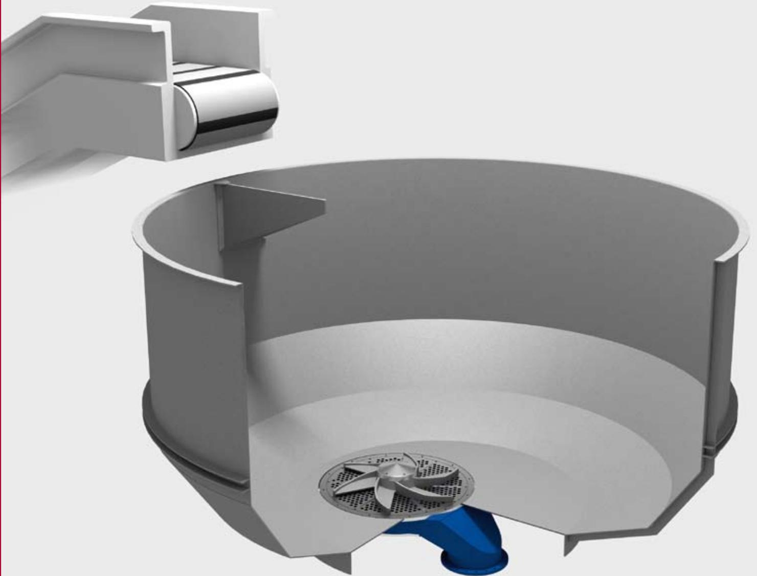
*IntensaPulper IP-V with double break bottom tank and eccentric rotor.*
