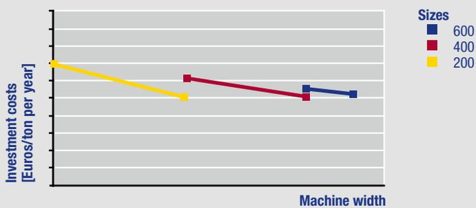
Fig. 3: One Platform Concept – Optimal investment costs for each size.
