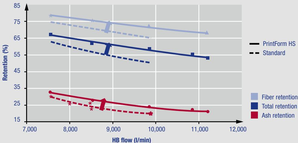
*Compared to standard fabric: Higher retentions with PrintForm HS and 10-40% less retention aid dosage.*
