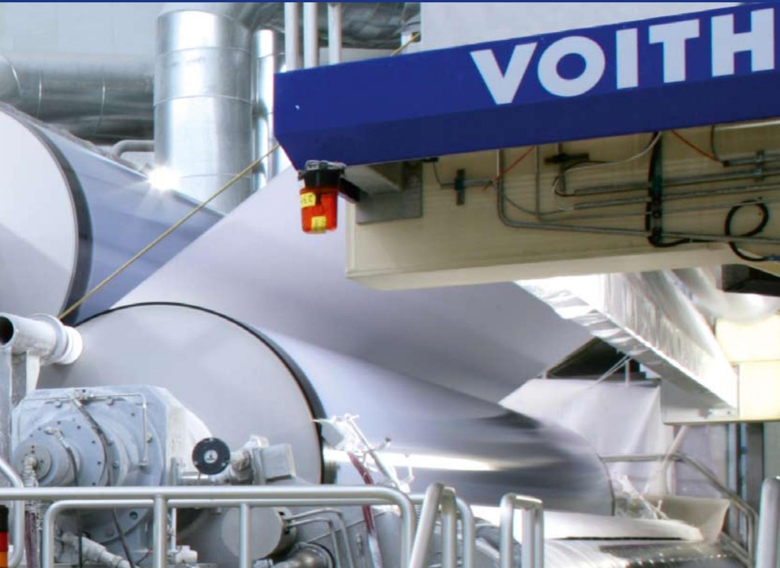
*SpeedSizer film press with Luna roll covers provides a constant film coating process.*
