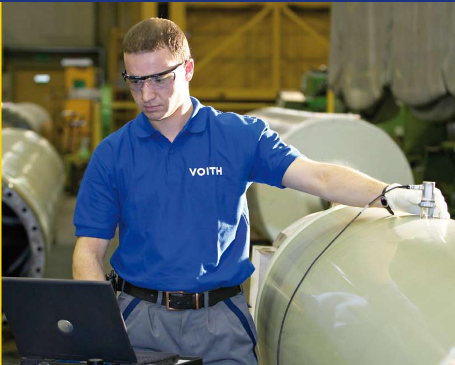
*RollCare: Ultrasonic testing of a roll cover.*
