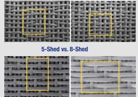
Open warp structure and sheet support mechanism.
