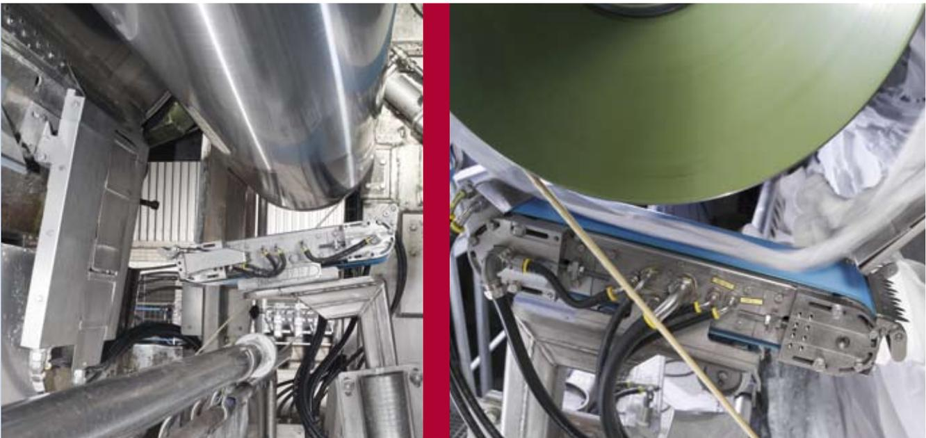
Fig. 4: Prevo threading solution on the PM in the SpeedSizer section (left: operating position; right: successful hit).
