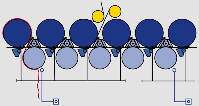
*SafeTailing in the TopDuoRun dryer section – tail cutting with pushbutton or with controller by means of vacuum sensor.*
