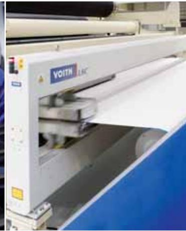
Fig. 3: The Voith LSC Scanner checks paper quality.
