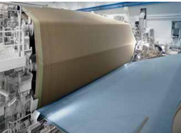
Fig. 1: Wire section and pick-up felt.
