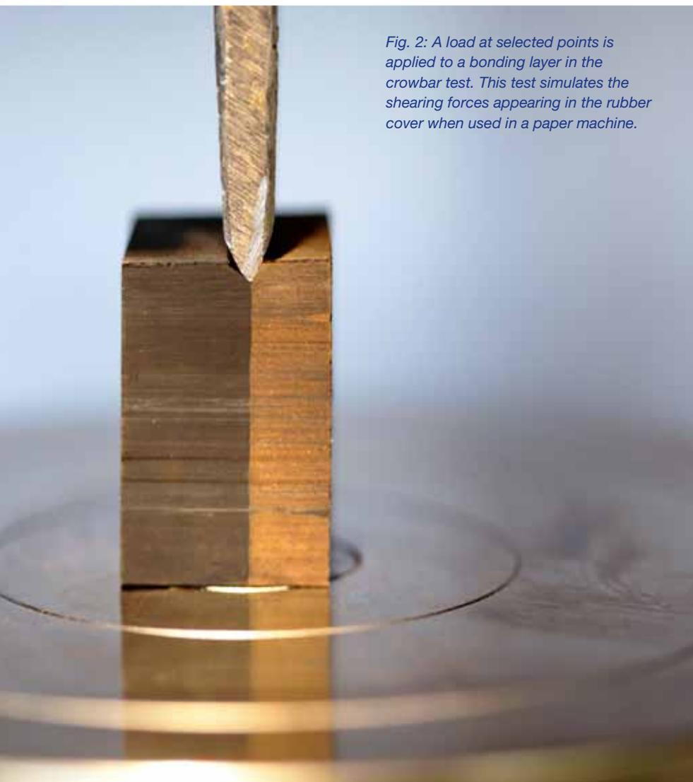
*Fig. 2: A load at selected points is applied to a bonding layer in the crowbar test. This test simulates the shearing forces appearing in the rubber cover when used in a paper machine.*
