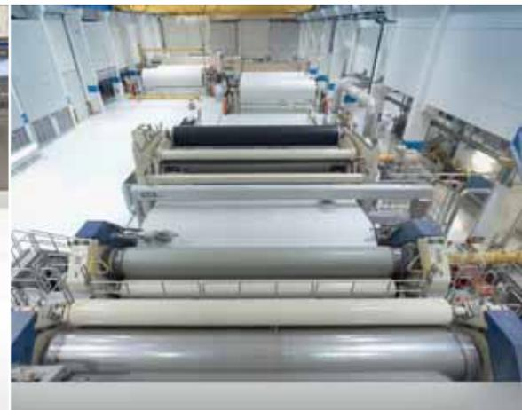
Fig. 3: Various roll coatings and covers in the finishing area.
