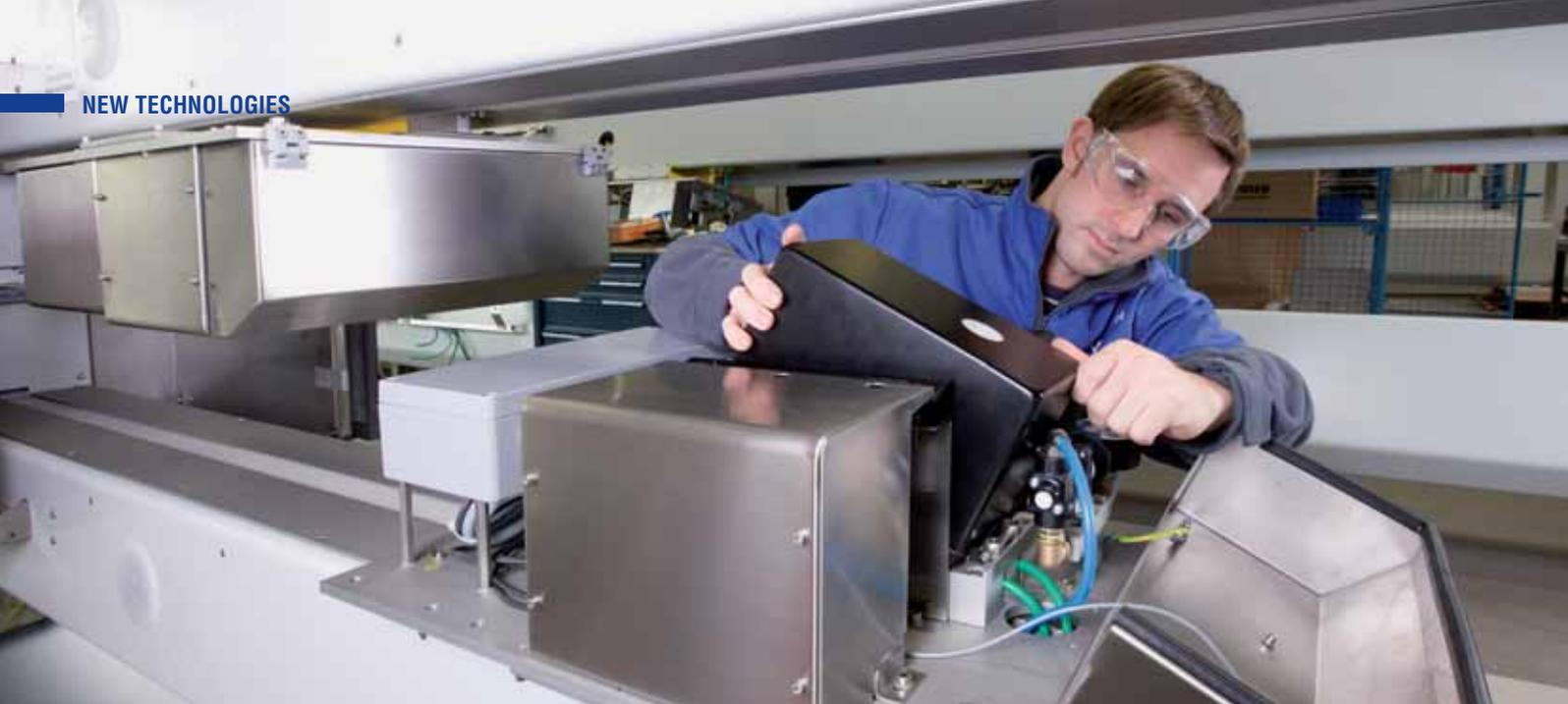
*Fig. 1: A Voith technician installs and tests the Voith LSC TecoScan system in the factory.*
