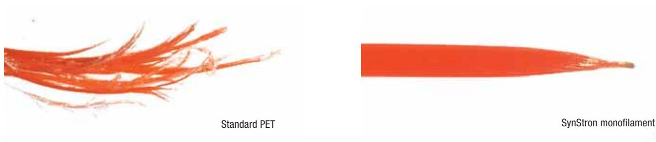
Fig. 4: The SynStron yarn filament is less prone to fibrillation. In contrast, the standard PET filament (left) has numerous small fibrils after a sudden break.
