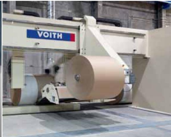
Fig. 2: Mobile-mounted winding head of the ClassicPlus roll packing machine.
