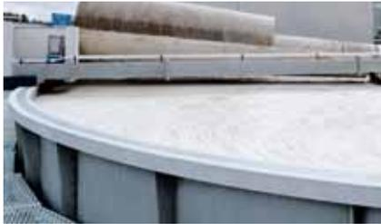
Anaerobic reactor technology in combination with a lime trap makes the lime problem manageable. It enables biologically treated and decarbonized water to be recirculated into the production process. This recycling lowers the average water consumption in paper production.
