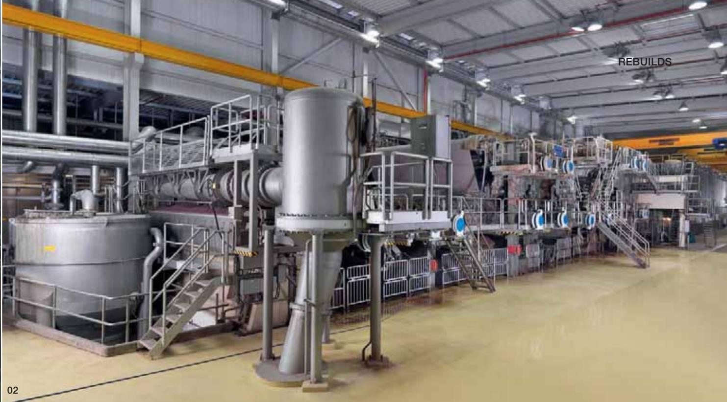
Fine screening in all lines was fitted with MultiFoil rotors and C bar Q screen baskets, and the centralized fiber after-treatment was equipped with the latest generation of refining fillings. This has resulted in an exemplary overall solution that is both technologically sophisticated and economical. Line 1 has been in operation successfully since July 2011. Lines 2 and 3 started up in March and July of this year.
