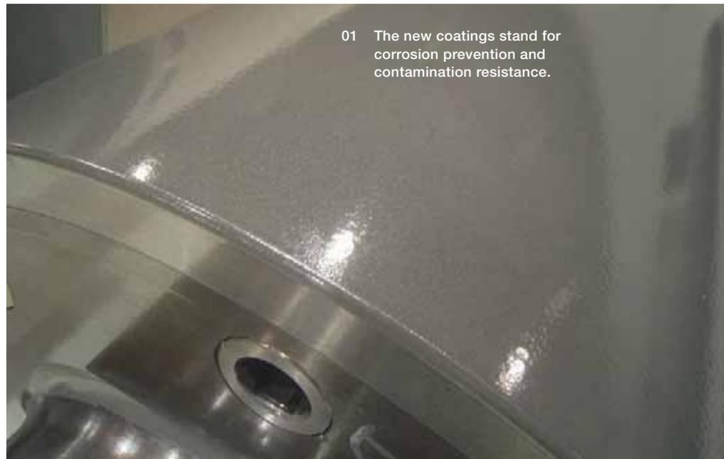
01 The new coatings stand for corrosion prevention and contamination resistance.
