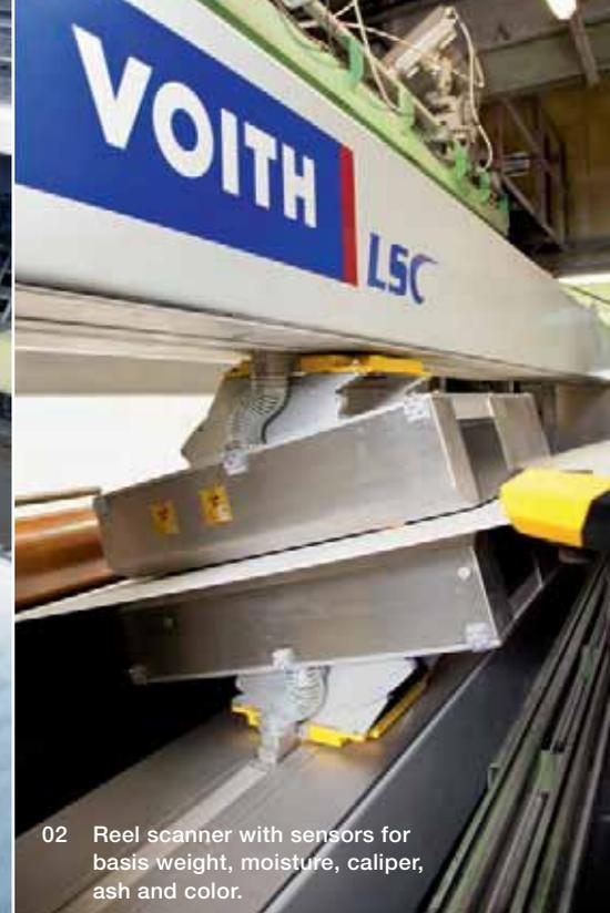
02 Reel scanner with sensors for basis weight, moisture, caliper, ash and color.
