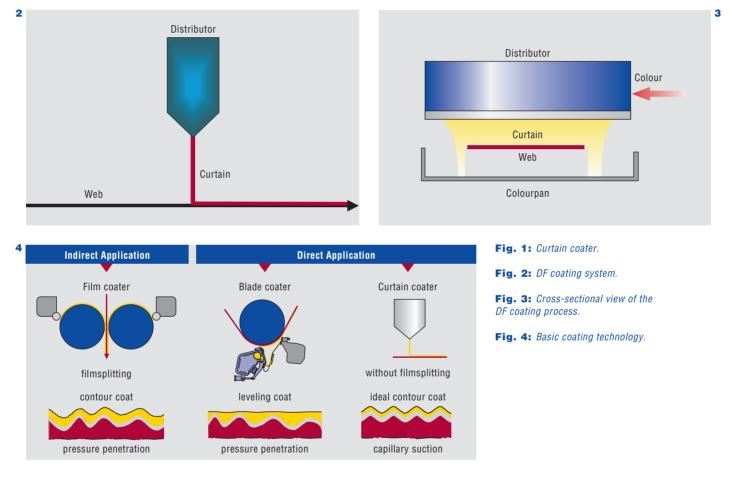
Curtain coating (Figs. 1 and 2) is a relatively new process with very high efficiency, good coating quality, easy operation, cleanliness, etc. So far, this type of coater was hardly used in paper production, because of difficulties in controlling the air boundary layer on the web, coating color deaeration and curtain stability.
