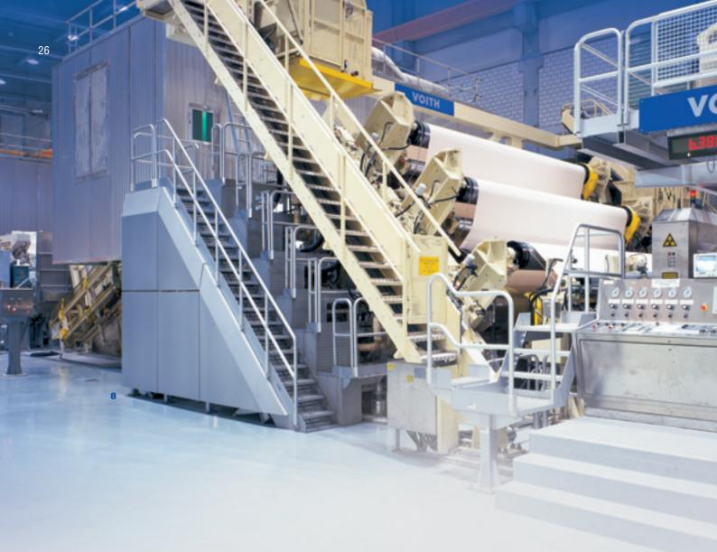
here, up to paper roll diameters of 3,200 mm and with minimal waste, is ensured by a Sirius<sup>™</sup> reel system at the end of the line.
