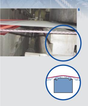
The air-hood shown in **Fig. 7** features nozzles specially designed for the paper industry and can, in connection with an air heating device, be used as a stand alone system (CB-Dryer) for LWC grades (3 recent installations in the US), high quality coated paper (Propal/Columbia) as well as for virtually all other paper grades as has been proven many times in the pilot coater of the PTS in Munich.
