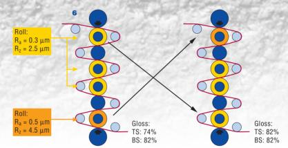
**Fig. 6:** Effect of soft roll surface roughness on calendering results.  $v = 1,000 \text{ m/min}, Q = 450 \text{ N/mm}, T = 130^{\circ}\text{C}$ coated wood-free paper, calendered on both sides, 100 g/m<sup>2</sup>
