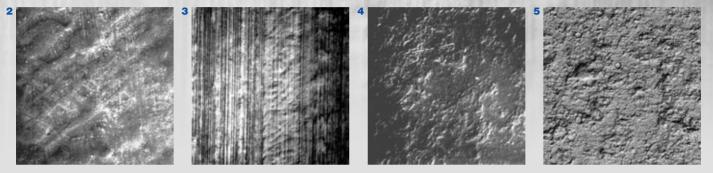
The steel or grey cast iron rolls used in the first supercalenders wore out so rapidly that they soon had to be replaced by chilled cast iron rolls. The impression of such a roll surface in **Fig. 2** clearly shows the roughness due to the relatively coarse iron carbide microstructure.
