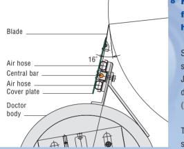
Fig. 8: Doctor blade arrangement.
