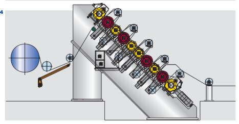
hand the CD thickness profile is optimized, which significantly improves runnability in the coating machine, and on the other hand moderate precalendering makes for more efficient calendering.
