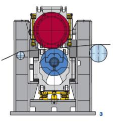
In these one-stack layouts, the two softcovered middle rolls form the reverse nip. To correct two-sidedness in such layouts, different temperature settings are required above and below the reverse nip.
