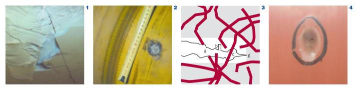
the temperature rise causes cover expansion mainly in the radial direction. This process is repeated with every nip pass. The sum effect of periodic overloading and thermal expansion is a self-energizing cycle, which even might continue after the initial pulse due to roll deposits ceases.
