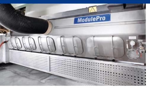
The ModulePro C jet spray dampener moistens the paper web in the coating machine.
