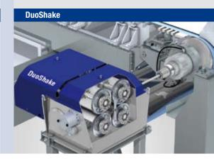
For décor paper machines Voith Paper uses the MasterJet headbox in conjunction with the EdgeModule edge feed-in system to achieve optimum fiber orientation at the web edge. The DuoShake shaker ensures a particularly homogeneous distribution of the fibers in the sheet.
