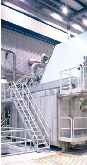
liquid curtain to the paper web. In order to reduce curling that occurs for papers with one-sided coating (warping in the paper), each of the two coating machines were equipped with a ModulePro C jet spray applicator system in 2006. The ModulePro C compensates for the roll tendency of the paper by releasing frozen warps that remoisten the web on the non coated side. The new technology
