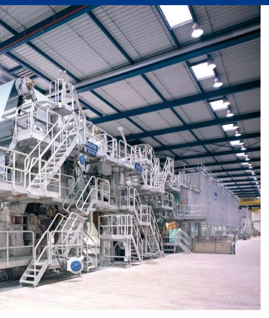
The PM 2 at the Koehler facilities in Kehl is used exclusively for the production of thermo papers in the basis weight range of 40 to 80 g/m² and at a production speed of 1,600 m/min.
