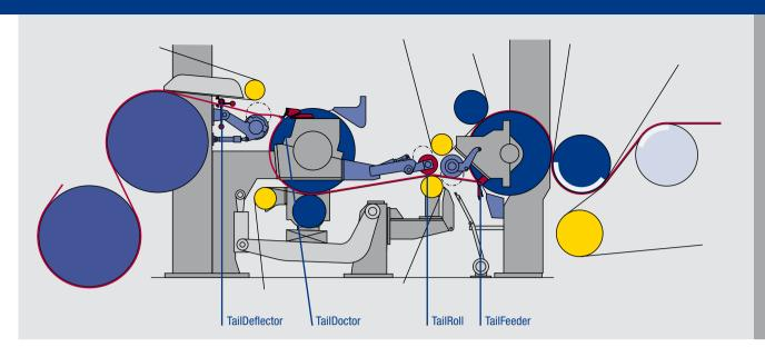
The "Value Plus Thread Concept" (red marking) is suitable for retrofitting in existing specialty paper machines.
