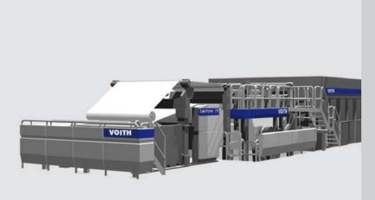
In a special Voith Paper machine for banknote paper, the MasterVat and ShortFormer B are used for the double-ply sheet forming.
