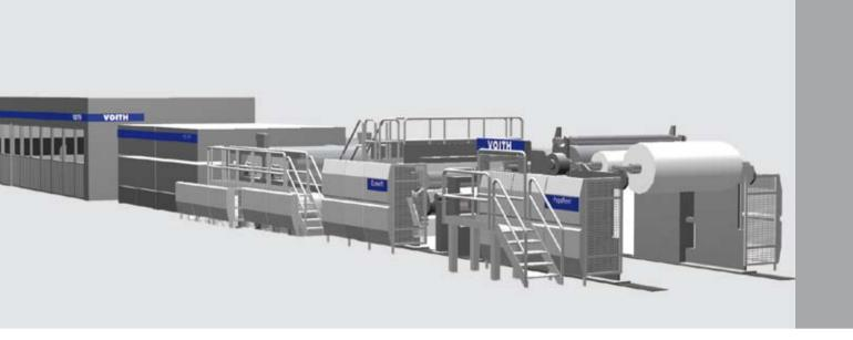
embedded into the paper. Both of these authenticity attributes are worked into the paper during the forming section of the machine. The double-layer forming system from Voith Paper, which consists of the Master-Vat and the ShortFormer B, makes Voith the market leader in this technique. Nearly all European banknote paper mills produce the second paper layer using the Short-Former B that Voith Paper has continued to develop.
