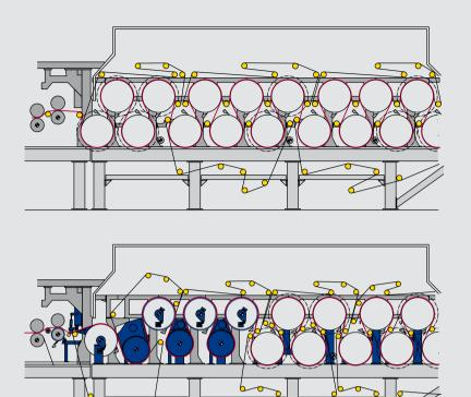
Before the rebuild by Voith Paper, the paper machine in Besozzo was a fourdrinier machine with dandy roll producing décor paper. The rebuild now makes it possible for the PM 4 to produce masking tape as well.
