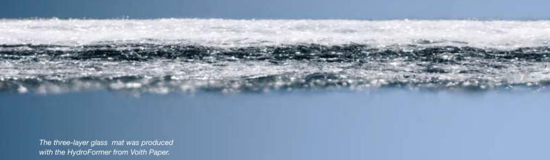
Glass fiber mats are used as the base material for floor coverings, asphalt shingles and asphalt rolls, among other products. There are older glass mat machines operating in the width ranges of 2 to 5 meters. But to achieve higher production capacities the latest installation is the largest glass mat machine in the world. The formation width of the new machine is 5,300 mm with production speeds of over 400 m/min.
