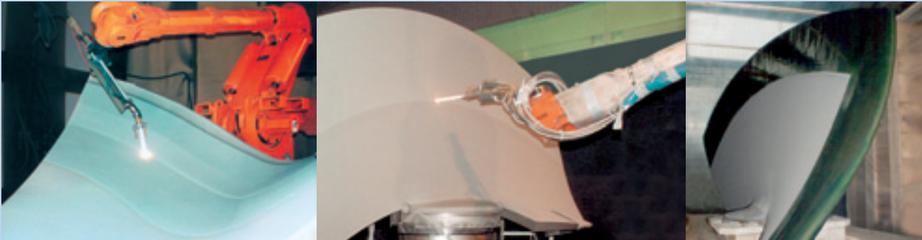
Application of the Diaturb® 532 coating
