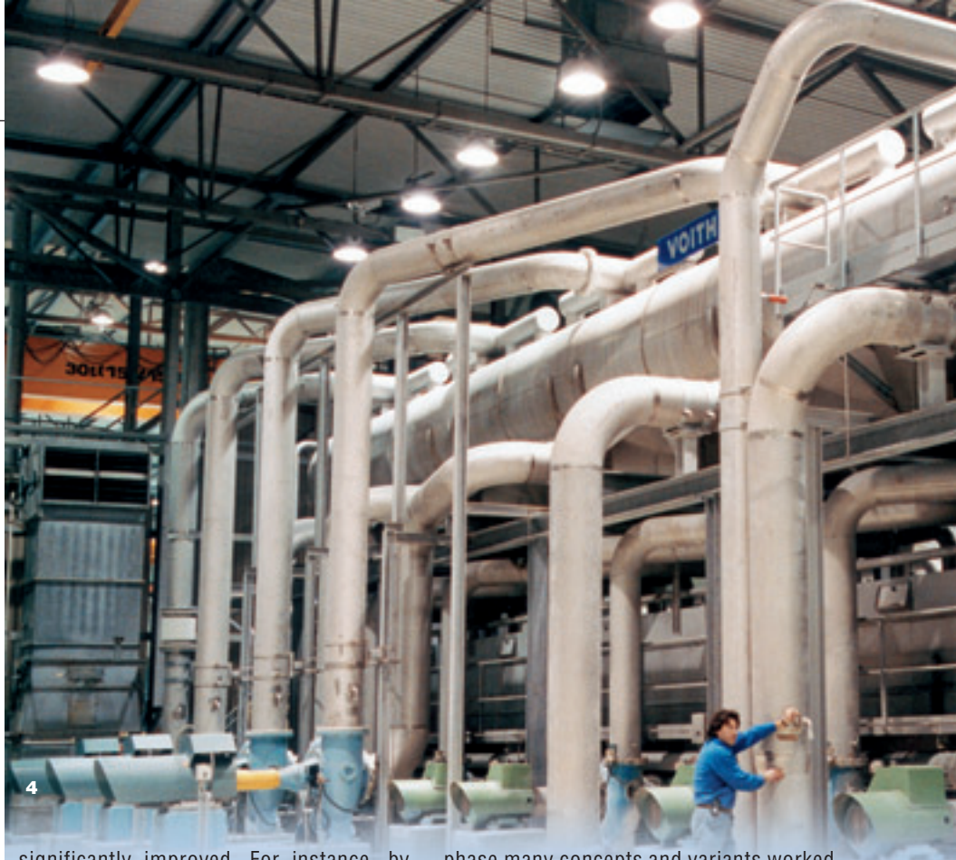
Fig. 4: The existing RCF1 plant was extended by an EcoCell flotation deinking line in the new Loop 2.
