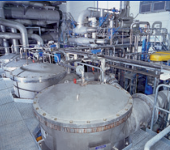
MultiSorter coarse and MultiScreen fine screening, with C-bar baskets and Multi-Foil rotors.
