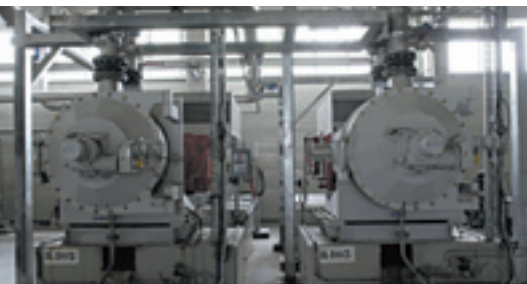
TwinFlo double disc refiners for refining the long fibers.
