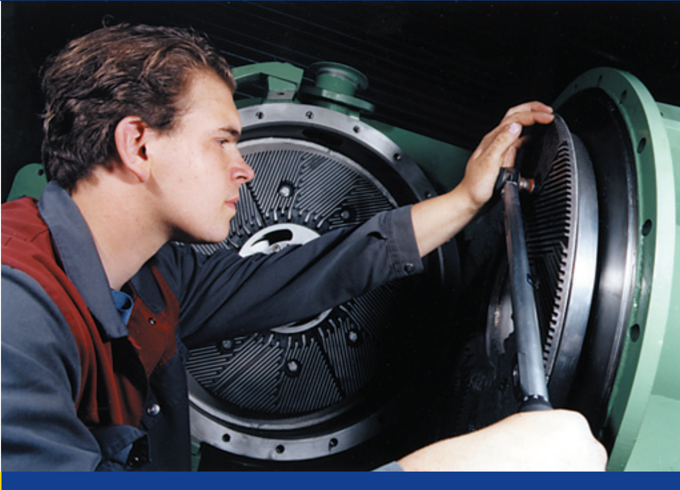
Exchanging the refiner fillings of a TwinFlo TF1D double disc refiner.
