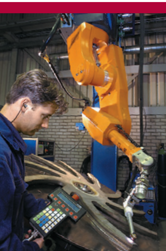
Robot welding technology for repairing rotors.
