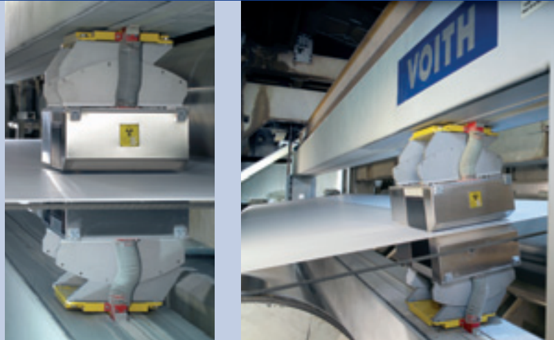
The OnQ Scanners incorporate sturdy box-frame construction that provides inherent dimensional stability.
