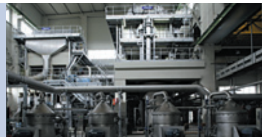
Thune disc filters for thickening (background) and the final stage LC slot screening for the long fibers (foreground).
