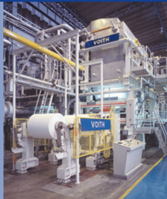
Tissue pilot machine at the Voith Process Technology Center in São Paulo.
