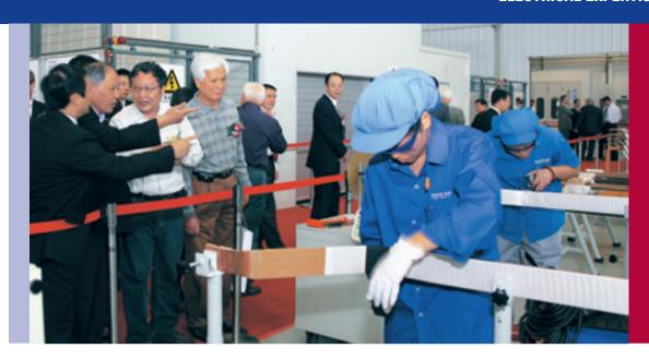
During the opening festivities in Shanghai, employees demonstrate insulation of stator bars which is the heart of stator bar manufacturing.
