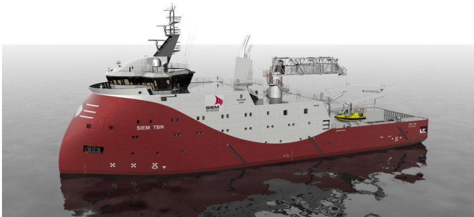
The Siem Moxie: First infield support vessel with the X-Bow Design and with Voith drive system.
