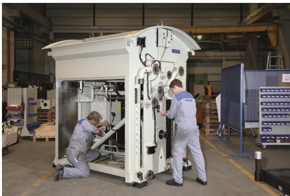
Caption 3: Assembly of the cooling system for high-speed trains (HST) Class 43.
