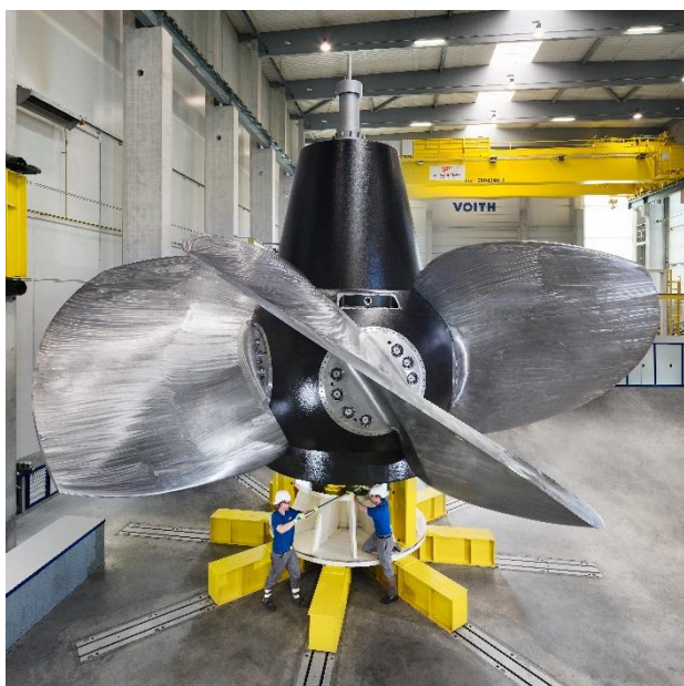
Caption 2: A vertical Kaplan turbine for the Russian hydropower plant Saratov weighs 314 metric tons.
