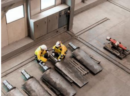
VSP blades during the overhaul in the workshop.
