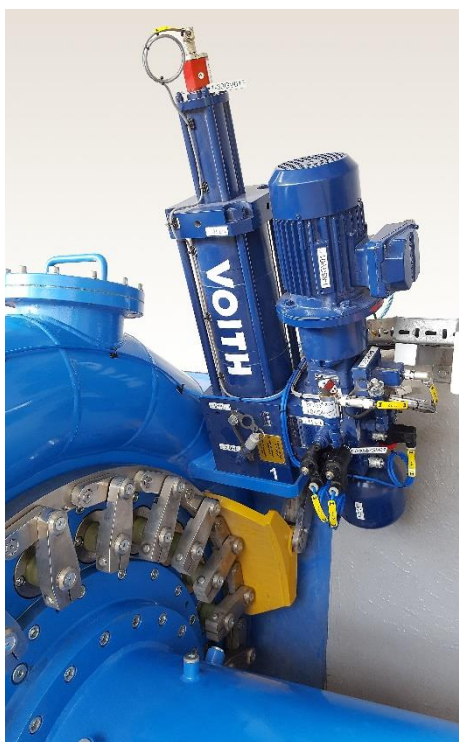
Caption 2: The new turbine control unit regulates the water flow by adjusting the turbine blades.
