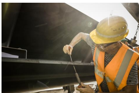
Caption 1: BeltGenius ALEX analyzes the alignment of carrying idlers in conveyor systems and reports the problem to mine operators.
