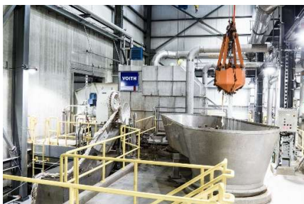
Pulper unit within the stock preparation
