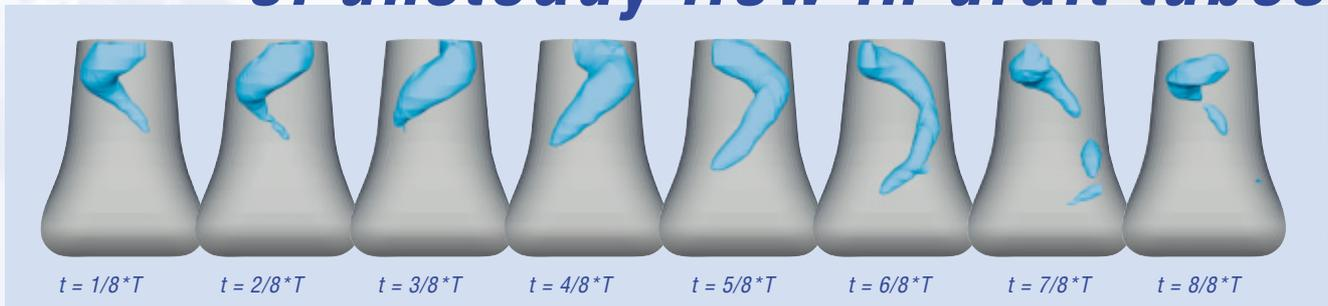
Calculated vortex rope at different times.
