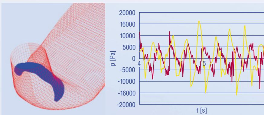
*Bifurcating cavitating vortex rope in the model test stand.*
