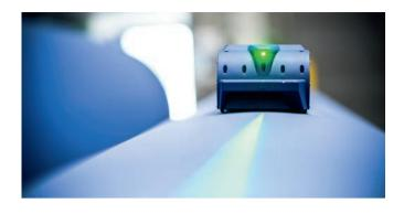
The Voith Surface Scanner is a self-driven device with a laser measuring head. It provides seamless full-width measurement and photo documentation. The data transfer works easily via an SD-card to a laptop for analysis. The self-driven Surface Scanner is aligned by a laser head and follows a straight line without any pushing or holding, thereby measurement irritations are eliminated.
