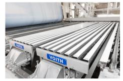
By individually setting the height and angle, VForm can be used to adjust the fiber suspension for the specific grade. This increases e.g. the dewatering capacity and improves the strength of the paper.
