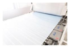
At the Schönfelder Papierfabrik PM 1, three conventional boxes have been replaced by two VForm hydrofoil boxes. By using the VForm hydrofoil,
