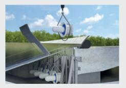
Illustration of StreamDiver in the hydropower plant.
