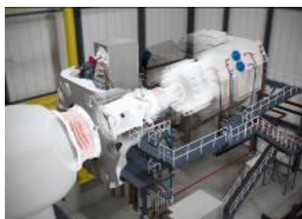
A Voith SafeSet coupling protects the DyNaLab from damage in case of an incident during test runs. (Source: IDOM)
