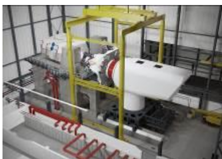
Fraunhofer IWES operates the large-scale test system DyNaLab for wind power nacelles in Bremerhaven, Germany. (Source: IDOM)
