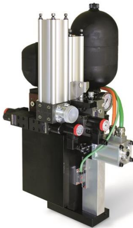
Caption 2: Hydraulic Stroke control for punching machines with DECV Valve. The cycle time at a stroke of 4 mm is 18 ms.
