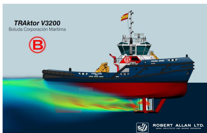
Caption 2: Thanks to the VSP propulsion system, the multi-purpose tugs designed by Robert Allan can be maneuvered precisely, even out at sea.
