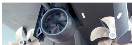
VIP1000-300 as swing-out auxiliary propulsion unit.
