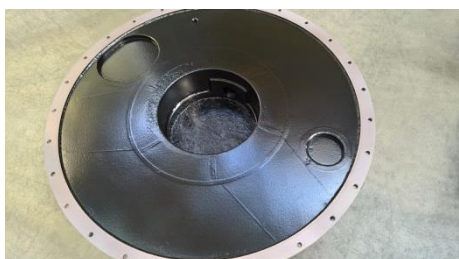
Coating of a housing base while it is being overhauled.
