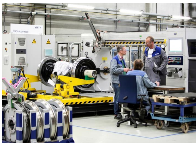
Caption 1: The wheel set press is part of the bogie shop at the Voith Rail Service Center where different processes are integrated under one roof.
