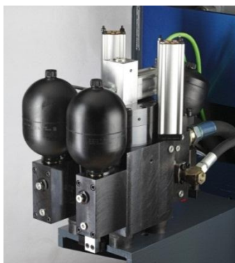
Figure 4: The HPPC electrohydraulic high-performance punch drive achieves over 1 500 cycles per minute.
