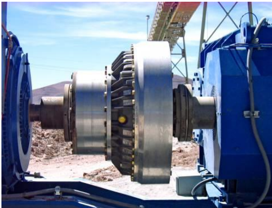
Photo 1: The Voith constant-filled fluid coupling protects the components in belt conveyor systems, increasing their availability.
