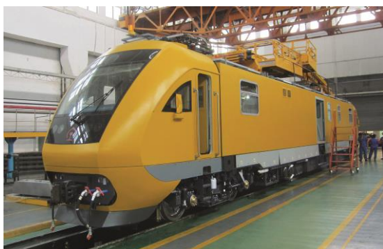
Special rail vehicle for overhead wire inspection, type BR 711 CN, drives with Voith turbo transmissions
